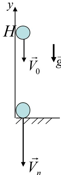
$$\begin{cases} V_y = V_{0y} + g_y t \\ \Delta r_y = V_{0y} t + \frac{g_y t^2}{2} \end{cases}$$
