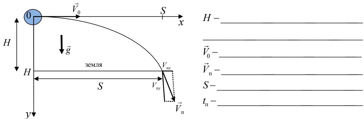
$$\begin{cases} V_x = V_{0x} + g_x t \\ x = x_0 + V_{0x}t + \frac{1}{2}g_x t^2 \end{cases} \quad \begin{array}{l} V_{0x} = \text{_____} \\ V_{0y} = \text{_____} \\ g_x = \text{_____} \end{array}$$
