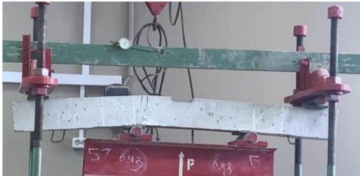
Figure 2 – The diagram of the beam in the experimental installation after the destruction of the normal section
