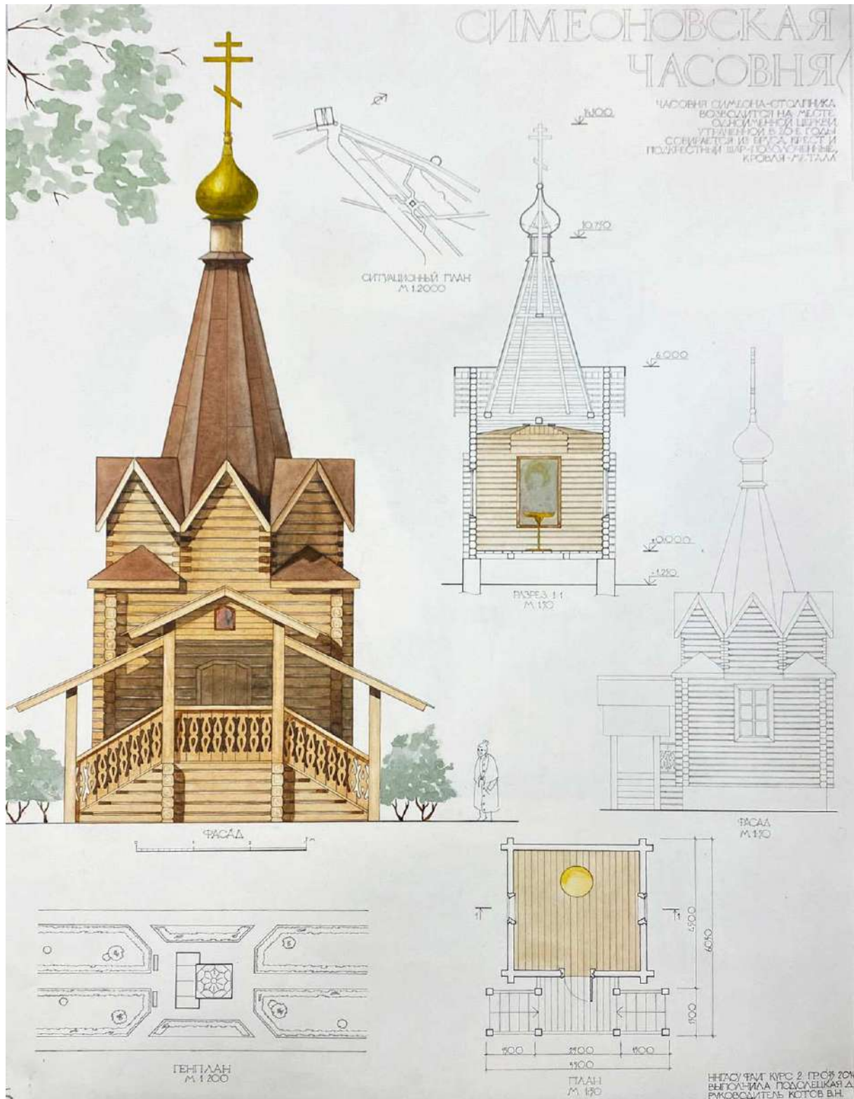
Fig. 66 An example of a graphic design for a chapel project made from rounded logs.
