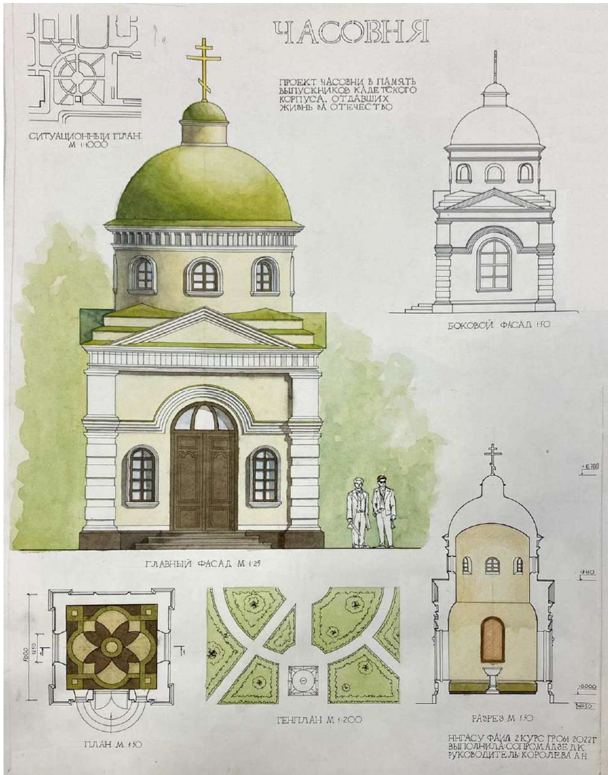
Fig. 68 An example of the graphic design of a chapel project in the neoclassical style.
