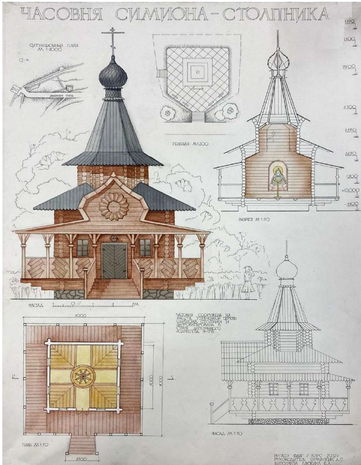
Fig. 67 An example of the graphic design of a chapel project made of rounded logs with a walkway.
