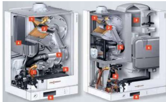
Figure 3. The construction of a condensing boiler (Viessmann Vitodens 100) running on gas fuel: 1 - heat exchange surfaces, 2 – modulated cylindrical burner, 3 – capacitive storage, 4 – expansion tank, 5 – burner fan, 6 – pump, 7 – plastic heat exchanger for hot water, 8 – liquid crystal touch screen display
