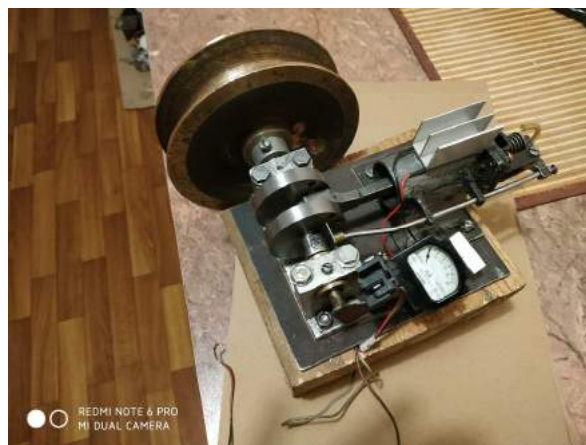
Figure 1. Lenoir engine with added Peltier elements
