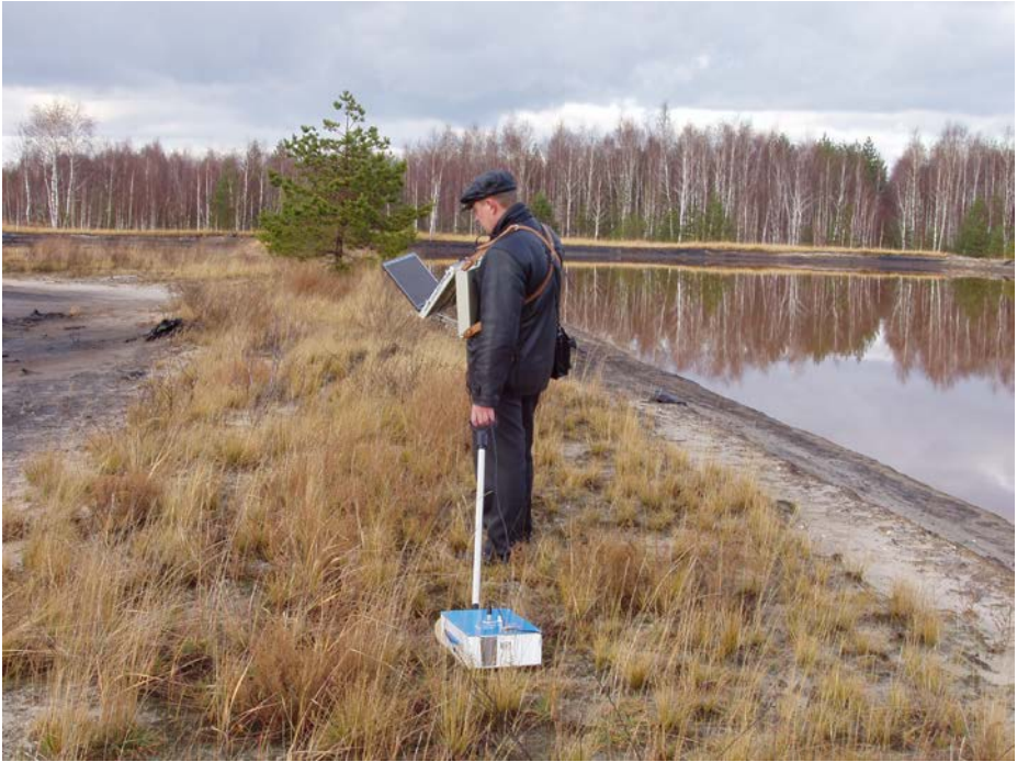
Fig. 4.28 Georadar tar ponds longwise profiling
