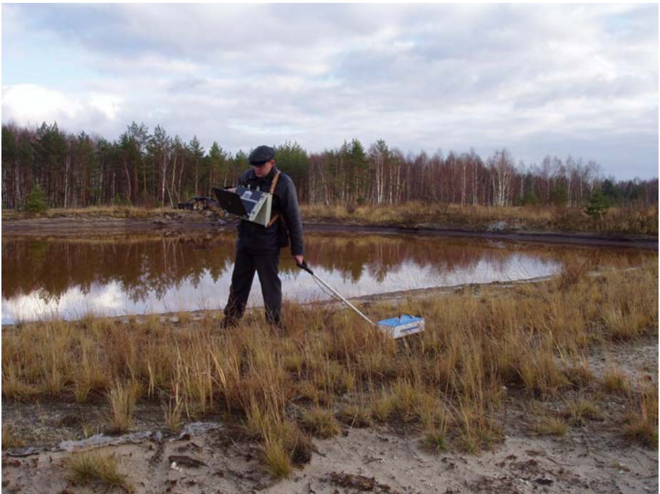
Fig. 4.29 Georadar tar pond crosswise profiling
