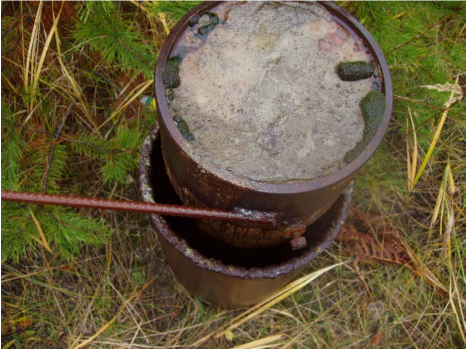
Fig. 4.31 Observation well used for tracer testing in the area of acid tars
