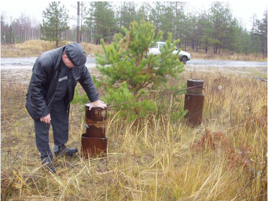
Fig. 4.32 Observation wells used for fluorescein injection
